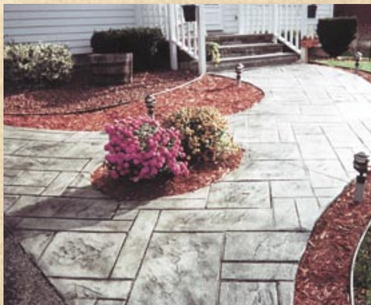
Silver Integral color and Charcoal Release were used with the Random Slate design to create this breathtaking sidewalk.
